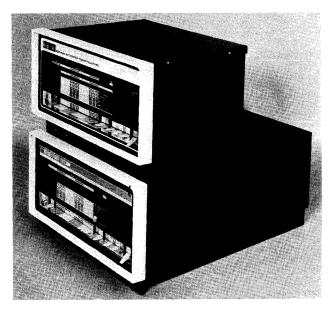
The PDP-8/E (on the bottom) is the most powerful in a long and extremely popular line of 12-bit minicomputers from DEC. It features a patented internal bus system called "Omnibus". DEC also offers a lower-priced, modular version called the PDP-8/M (perched above) for OEM customers.
