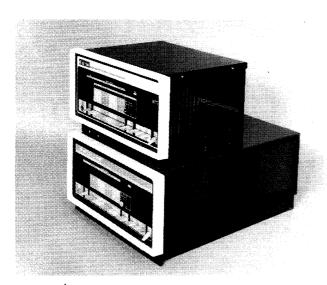
The PDP-8/E on the bottom is the most powerful model in the long and extremely popular line of 12-bit minicomputers from DEC The PDP-8/M perched above it is a lower-priced modular version for OEM customers.
