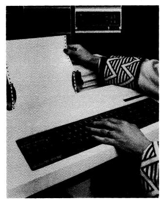
The PDP-11/70 represents the high end of one of the most extensive minicomputer product lines in existence today. The PDP-11/70 is a high-performance machine with integral cache memory and high-speed 32-bit data paths. The system also has memory management, look-ahead, and internal memory expansion capability up to 4096K bytes.
