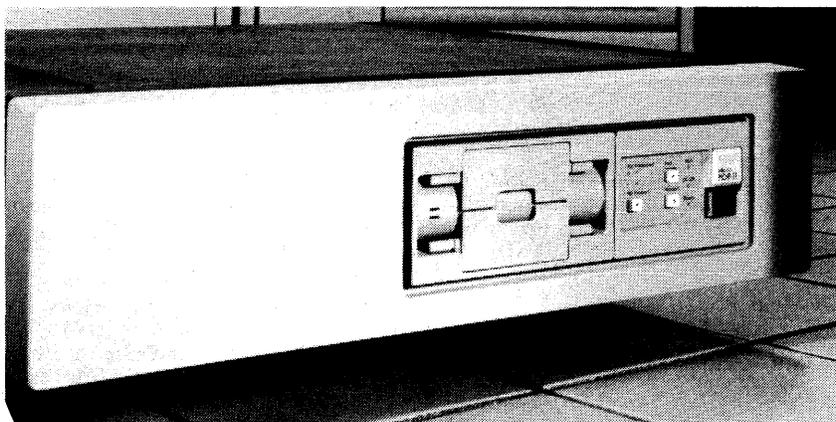
*DEC's Micro/PDP-11, based on the PDP-11/23-PLUS, combines CPU, memory, 10.8MB of disk storage, controllers, and power supply in one 5¼ inch high box. The Micro/PDP-11 system is a full-fledged PDP-11 processor with 22-bit addressing capability and runs standard PDP-11 operating systems such as RSX-11M-PLUS, RT-11, and RSTS.*
