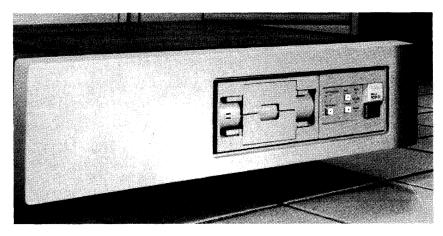
The Micro/PDP-11 is the low-end system in DEC's PDP-11 family. Based on the PDP-11/23-PLUS CPU, the Micro/PDP-11 supports from 256KB to 4MB of main memory and 10MB to 38MB of mass storage. It can also control up to six concurrently active workstations. The Micro/PDP-11 can run such standard PDP-11 operating systems as RT-11, RSTS/E, and V7M-11 Unix, as well as Micro/RSX, a specially extended version of RSX-11M-Plus.
