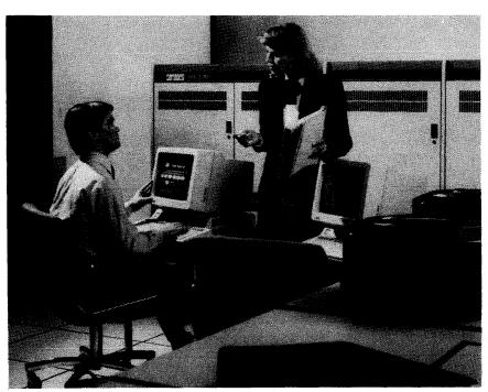
The VAX-11/785 is the high-end system in Digital Equipment Corporation's VAX-11 Systems family. The VAX-11/785 supports over 300 terminals, and, like other VAX-11 and VAX 8000 systems, can be configured in multiprocessor VAXclusters for enhanced storage and computational power.
