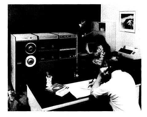
A typical single-user, interactive Datasystem 530 configuration is shown here. Based on DEC's powerful PDP-11/40, this system adapts well to small-business EDP environments. This particular configuration includes, from left to right, a 45-ips TU10 D magnetic tape unit, 4.8 million bytes of storage provided by 2 RK05 disk drives, a PDP-11/40 central processor with 16,384 words of 1-microsecond main memory, a VT05 CRT display terminal, and a 132-position LS-11 dot matrix printer.
