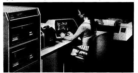
The PDP-11/40-based DEC Datasystem 530 shown here is a stand-alone, general-purpose small business computer, designed to provide single user batch capabilities under the Commercial Operating System (COS-500). The configuration shown includes a 64KB main memory, 4.8 million bytes of disc storage, a 300-cpm card reader, a CRT console, and a 132-position line printer.
