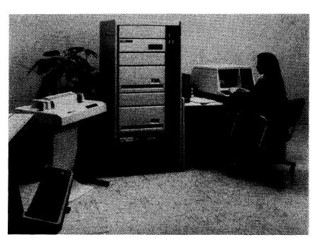
This Datasystem 325 configuration consists of a PDP-11/03 processor with 56K bytes of MOS memory, a cabinet holding dual RL01 removable disk drives with a total of 10 megabytes of on-line storage, a 4-line asynchronous serial interface, two DECscope consoles, and an LA180 printer rated at 180 cps. The price is \$34,500, including the CTS-300 operating system and DIBOL compiler.
