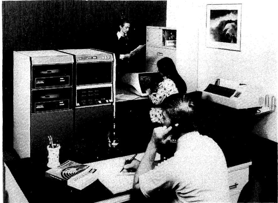
▷ above peripherals can also interface with the Unibus, and still work at their normal speeds. (The special PDP-11/70 fast bus and fast controllers for these peripherals serve only to assist the central processor.)
