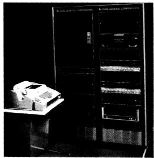
The new Dual Nova, which uses Data General's Real-time Disc Operating System (RDOS), is said to be the first dual-processor/shared-disc minicomputer available to users as a standard product. Three models are available, using a fixed-head Novadisc, a moving-head disc cartridge, or a disc pack drive. Prices start at \$44,930 for a basic Dual Nova 2 (pictured), and range upward to \$83,172 for a Dual Nova 840 sharing a 24.9-megabyte disc pack drive.
