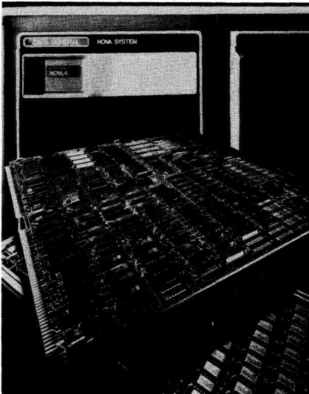
*The two-board design of Data General's Nova® 4/X computer incorporates CPU, MMPU, async interface, real-time clock, automatic program load, and power fail/auto restart on the CPU board, and up to 256K bytes of memory on a single memory board.*
