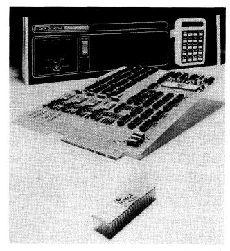
The microNova family is available in three basic configurations: chip sets, board computers, and fully packaged microNova minicomputers. All the packaged variations are built around the 40-pin mN602 NMOS microNova processor (foreground), which features a full 16-bit Nova architecture and main memory addressing capacity of up to 64K bytes.
