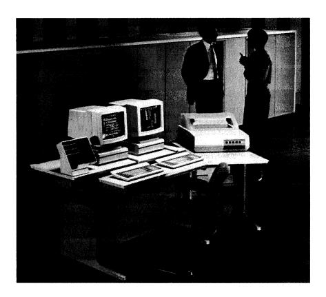
Bull's newest mainframe line, the DPS 9000 Series, is targeted for high-volume transaction processing and data management but can simultaneously execute numeric-intensive Fortran programs with its integrated vector processor. Shown is the Model 92T dual-processor configuration.
