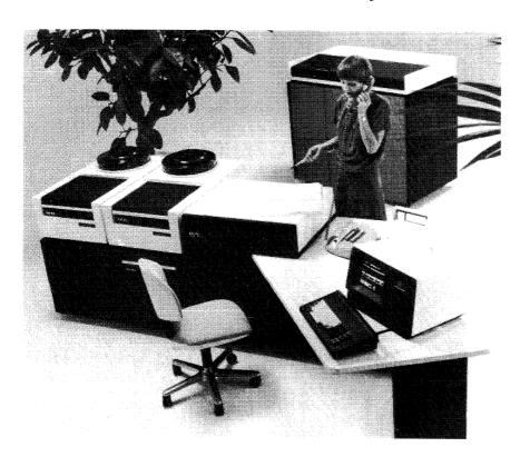
This large 61/DPS system includes three disk drives with a total capacity of 172.8 megabytes, the main enclosure containing the two processors with their associated memories and an integrated flexible disk drive, an 800 lpm system printer (rear), and the central workstation with a 2,000-character display and detached keyboard. This configuration can support up to 16 local or remote workstations and printer terminals plus synchronous communications.
