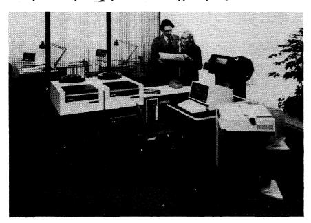
The small size of Cii Honeywell Bull's DPS 4 multiprocessor computer, its modular construction, and ease of operation make it a system as much for the office environment as for the traditional DP department. Pictured left is a system with 240 megabytes of removable disk storage, video console, and two system printers. Visual display terminals can be seen in the adjoining office area.
