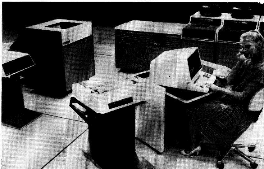
The new DPS 7/40E entry-level model features two to six megabytes of main memory, two to four I/O channels, a CRT console and keyboard, a Service and Unit Record Processor, and a maintenance diskette. It also supports a variety of peripheral devices.
