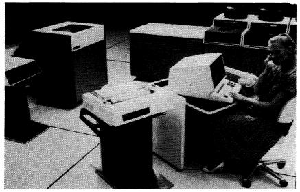
A typical small DPS 7 configuration includes the operator console and printer plus (from left) a diskette drive, high-speed line printer, the DPS 7/35E central processor, and three disk drives. The DPS 7 has from one to eight megabytes of memory and supports a wide variety of peripheral devices.
