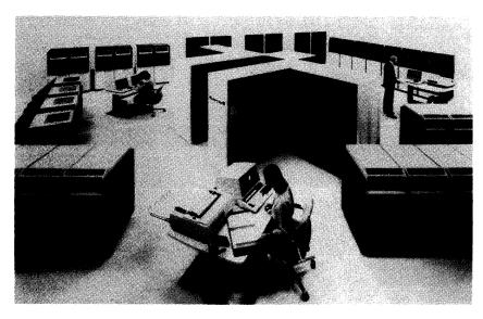
The DPS 88/82 shown here is a dual-processor system that can be configured with 128 megabytes of main memory and 128 channel function slots. As a networking/communications-oriented system operating within the Honeywell Distributed Systems Environment, the DPS 88/82 can support as many as 320 satellite processors in a variety of network structures.
