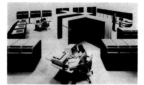
The DPS 88/82 shown here is a dual-processor system that can be configured with 128 megabytes of main memory and 256 logical channels. As a networking/communications-oriented system operating within the Honeywell Distributed Systems Environment, the DPS 88/82 can support as many as 320 satellite processors in a variety of network structures.
