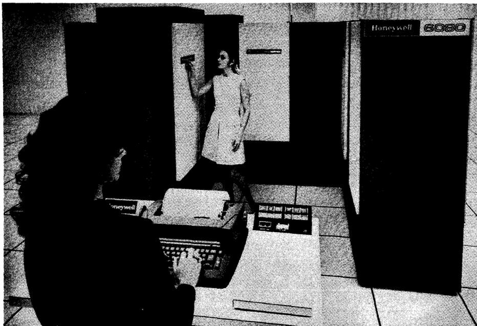
*Model 6080 is the most powerful of the six processor models in the Honeywell Series 6000. The Master Console is in the foreground.*
