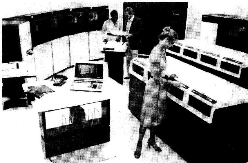
The DPS 8/20 is the smallest in a family of large-scale communications-oriented processors offered by Honeywell. They feature several operating systems, a wide variety of peripherals, and the capability to handle simultaneous batch, RJE, transaction processing, and time-sharing activities.
