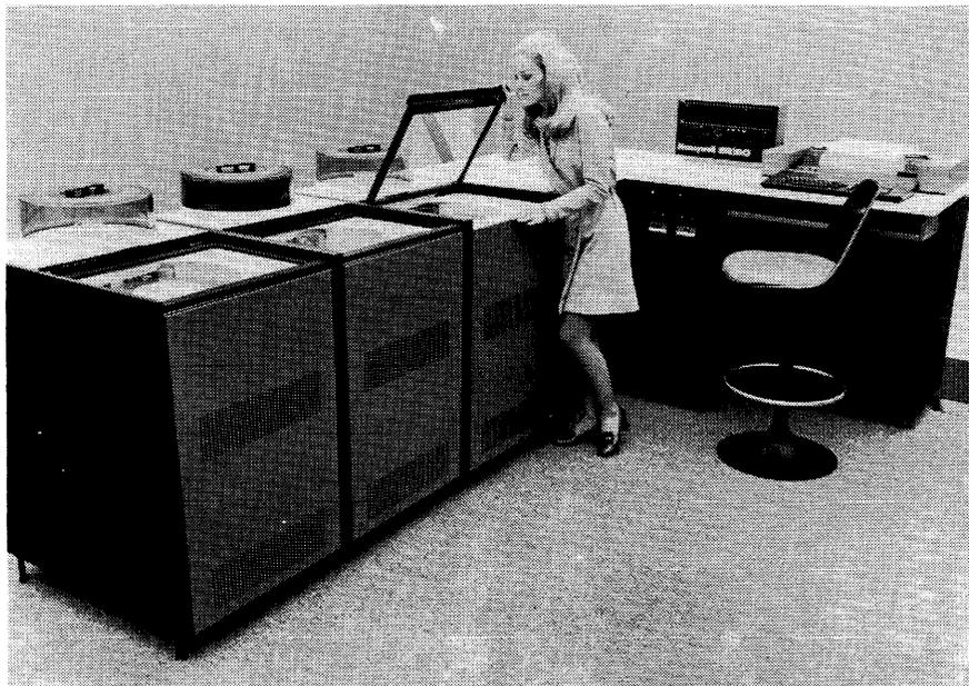
*The Model 62/60 is a small-scale disk-oriented system aimed primarily at attracting new users to the Series 60 product line. It offers from 65K to 131K bytes of 1-microsecond MOS memory. Typical system rental prices range from about \$3,500 to \$5,500 per month.*
