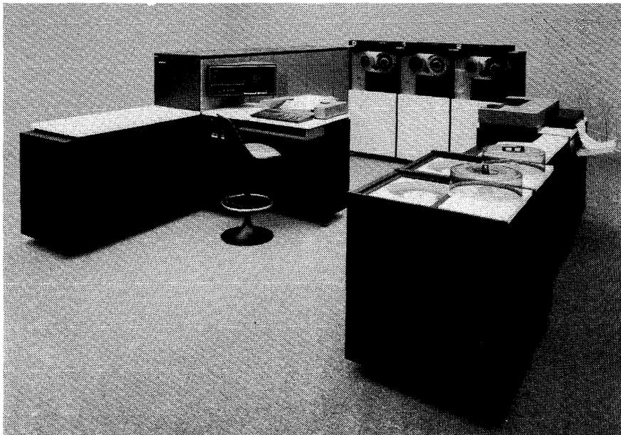
*The Model 64/20 features micro-programmed emulation of the Honeywell Series 200/2000 or Series 100 systems and is considered the logical upgrade system for most of the current small-scale installations in Honeywell's large customer base. System rental prices range from approximately \$6,000 to \$12,000 per month.*
