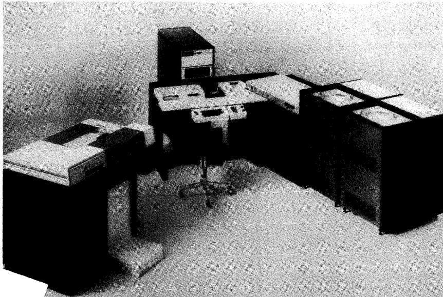
*The Honeywell Model 61/58 was introduced to the U.S. market in October 1974. Its basic configuration includes the central processor with 5,120 bytes of main memory, a dual-drive disk subsystem with 3.456 megabytes of storage, a 100-line-per-minute printer, and a 100-card-per-minute card reader console. This enhanced version of Honeywell's earlier Model 58 computer system can be purchased for \$66,590 or rented for five years at \$1,405 per month.*
