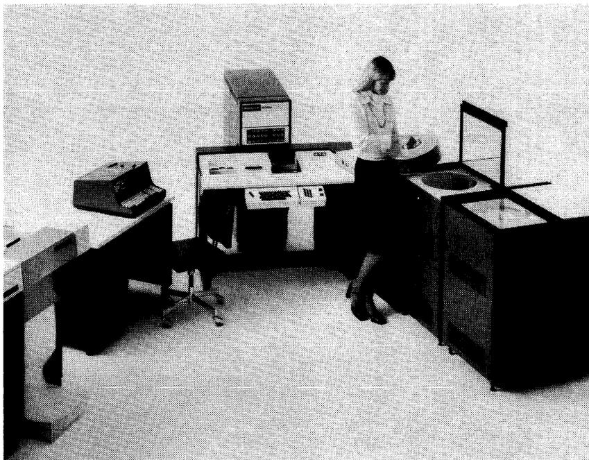
*The Model 61/60 Transaction Processing System in its minimum configuration consists of the central processor with 10,240 bytes of memory; a front-end processor with its related 8K-byte memory, CRT display, keyboards, and two cassette tape units; a 100-lpm, 128-position printer; a card console consisting of a 100-cpm card reader, numeric keyboard, alphanumeric keyboard, and 10-digit display; and a mass storage subsystem with 46 megabytes of disk storage.*
