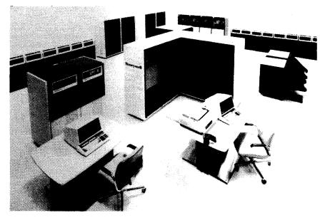
Honeywell's new DPS 88 family was developed in response to large users' increasing need for more processing power. Shown is the DPS 88/81 with up to 64 million bytes of main memory and 64 channel function slots. Automatic monitoring of system components and built-in fault and validation tests help ensure utility-grade reliability, availability, and data integrity.
