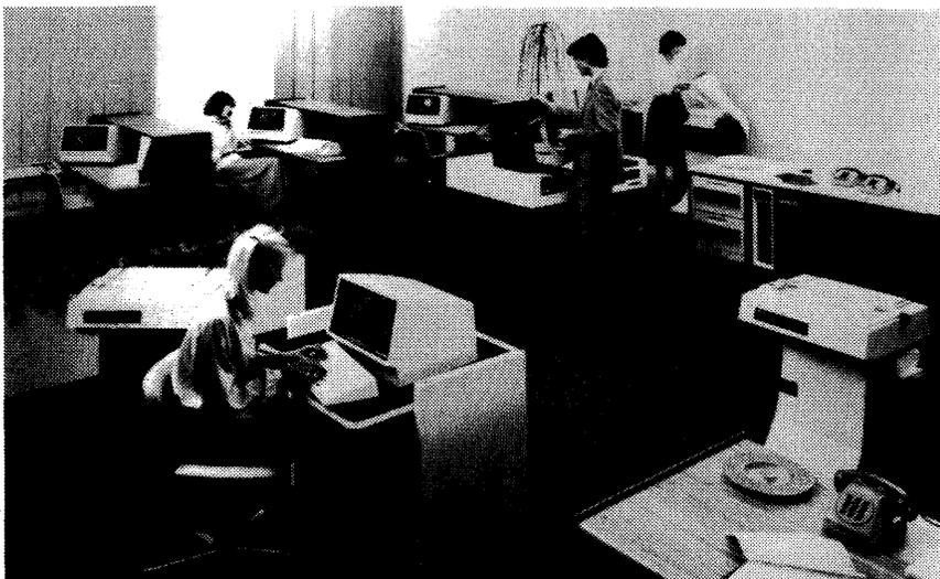
*For the larger user, Honeywell's DPS 4 computer can include up to a total of 12 processors. The picture shows a large configuration including double-sized central processor cabinet, 792 megabytes of removable disk storage, two printers, and visual display terminals—all operating in a normal office environment.*
