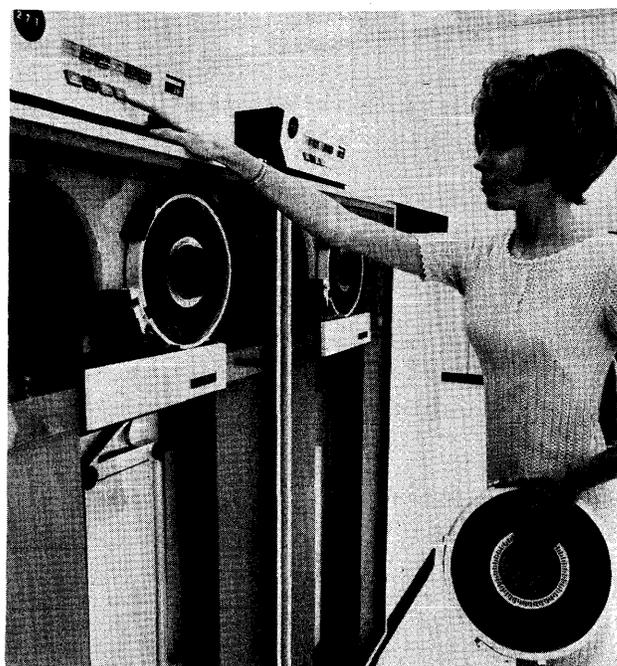
The IBM 3420 Magnetic Tape Units, introduced in November 1970, provide high performance (up to 320,000 bytes per second) at far lower prices than previous IBM tape drives.
