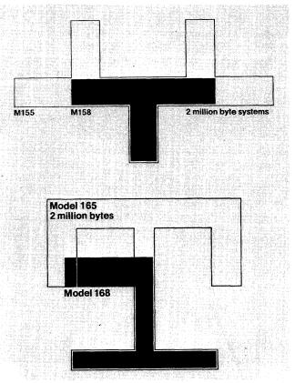
IBM's new MOS main memories result in greatly reduced floorspace requirements. The top illustration shows a 2-million-byte Model 158 CPU (shaded black) superimposed against a Model 155 with the same amount of core storage. Below, a 2-million-byte Model 168 CPU is similarly compared with a Model 165 of equivalent capacity.
