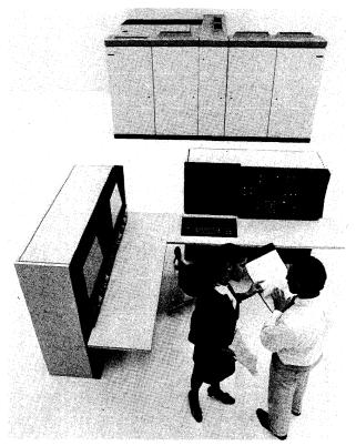
The Model 168, largest of IBM's virtual-storage computers, now offers up to 8 million bytes of real MOS main storage; a dual-processor 168 MP system can have up to 16 million bytes. The Model 168 console features a CRT display and keyboard.
