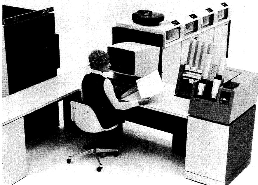
*The Model 115, the smallest and newest member of the expanding System/370 family, employs distributed processing techniques and features integrated control units for attachment of disk drives, magnetic tape units, card unit, line printer, and communications terminals.*
