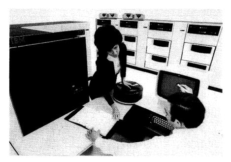
The Model 158 Processing Unit provides up to 4 million bytes of MOS main storage and is available in both uniprocessor and dual-processor (MP) configurations. A feature of the Model 158 is the CRT display console with light-pen input. An 8-drive 3330 Disk Storage subsystem is in the background.
