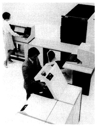
The Model 115, smallest and newest member of the System/370 family, employs distributed processing techniques and features integrated control units for attachment of disk drives, magnetic tape units, card unit, line printer, and communications terminals. Two 3340 Disk Drives are shown in the foreground, and the 3203 Printer is at left.
