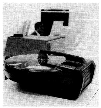
The 3348 Data Module, used in IBM's 3340 "Winchester" Direct Access Storage Facility, stores up to 35 million or 70 million bytes of data and combines the disks, access arms, and read/write heads into a single sealed cartridge.
