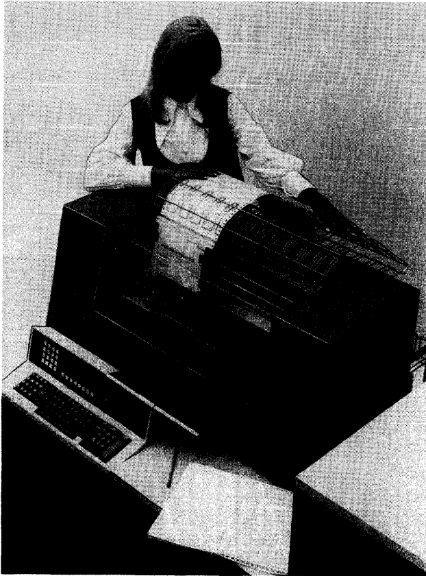
The wide-carriage 2222 Printer equips this System/3 Model 6 for ledger card processing. Cards up to 11 by 14 inches can be inserted into the feed slot (center).
