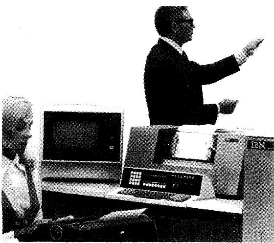
The optional 2265 Display Station complements the basic 5213 Printer at right by serving as a high-speed output device for the transaction-oriented System/3 Model 6.
