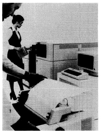
The System 34 is a member of the new wave of business computer systems packaged for use in standard office environments. Unlike the earlier IBM System 32, however, the System 34 offers a number of stand-alone peripheral devices, including both table-top and free-standing printers and a magnetic character reader.
