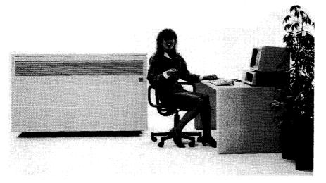
IBM's 4361 systems are targeted toward department-level computing functions in engineering/scientific and technical environments. The systems support up to 16MB of main memory and up to three high-speed block multiplexer channels for attachment of Direct Access Storage Devices (DASDs) and other high-speed devices. The three 4361 models run in IBM's proprietary DOS/VSE, SSX/VSE, VM, and OS/VS1 operating environments.
