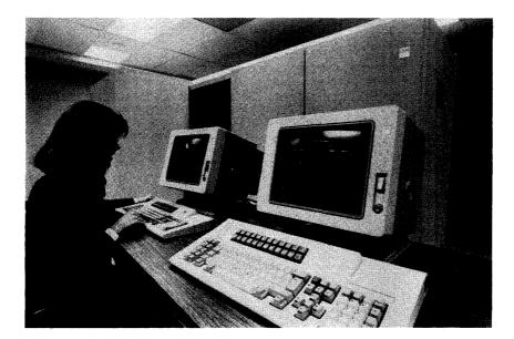
The IBM 3090 Model 200 dual processor, shown here, and the 3090 Model 400 four-way processor are IBM's newest top-of-the-line, largescale computer systems. They feature Emitter Coupled Logic and Thermal Conduction Modules, and achieve a cycle time of 18.5 nanoseconds.
