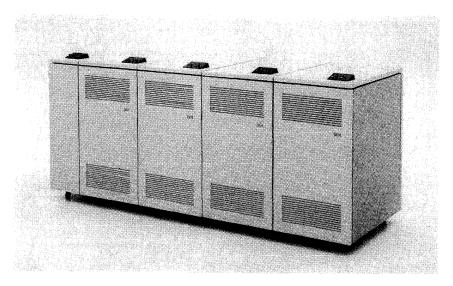
The IBM 3375 Direct Access Storage Device consists of up to four disk storage units. Each storage unit has a Head Disk Assembly (HDA) and two actuators, each actuator accesses 409.8 megabytes of data, a total of 819.7 megabytes per HDA.
