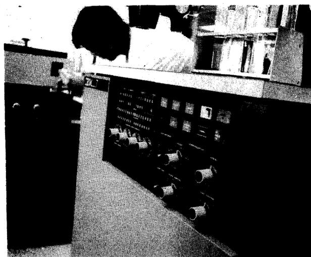
*The IBM System/7 can operate as a stand-alone system or in conjunction with other IBM computer systems in sensor-based applications that range from apartment house security control systems to telephone network controllers. Shown here as a laboratory automation system, the System/7 can handle readings from multiple measuring and testing devices.*
