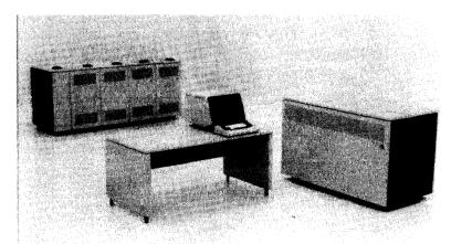
IBM's 4361 processor systems comprise Model Groups 3, 4, and 5. The 4361 systems are targeted toward department-level computing functions in engineering/scientific and technical environments. The 4361 systems can support up to 12MB of main memory, 241GB of online disk storage, and over 1,000 workstations. The three 4361 models run in IBM's proprietary DOS/VSE, SSX/VSE, and VM operating environments.
