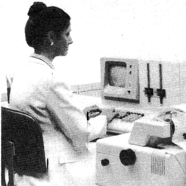
Dual integrated diskette drives and a larger display screen are the 5120's main functional advantages over its predecessor, the IBM 5110. In the foreground is the optional 5103 Printer.
