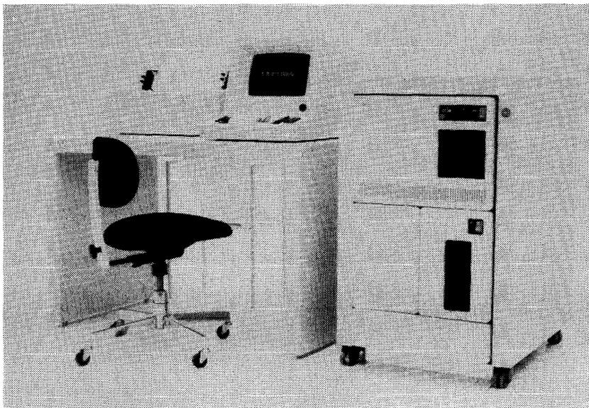
This small Series/1 configuration includes a low-boy rack enclosure housing the processor and a 4964 diskette unit. The table-top, 120-cps 4974 printer is shown at left. The display station in the photo is the 4979, one of two 1920-character-screen units offered with the Series/1.
