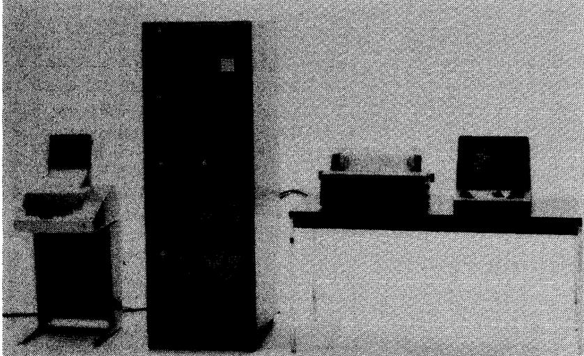
*This Series/1 configuration includes a 4997 rack enclosure with a 4955 processor mounted at the top and a 4959 input/output expansion unit below. The bottom half of the enclosure houses a 4962 disk storage unit, with a 4982 sensor I/O unit above and to the left, and a 4964 diskette unit to the right of the sensor unit. Also shown are the 4974 printer, 4979 display station, and a teletypewriter.*
