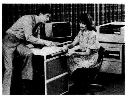
ICL's new System 25 includes a cabinet that contains processors, memory, a Winchester disc drive, and tape cartridge drives for software exchange. Also shown is a Model 85 visual display unit, one of several workstations available, and, at right, a fixed and exchangeable disc file.
