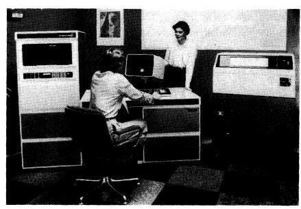
The ME29 range of medium-scale workstation-oriented systems offers extensive communications facilities. On the left is the processor cabinet which contains the central processor and either one or two floppy disk drives. A multi-purpose workstation is on the control desk, which also houses two 35MB fixed disk drives. On the right is a 600 lpm line printer.
