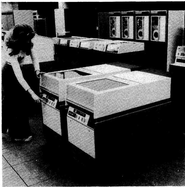
*Mass storage devices for the 2900 Series include the 100-megabyte EDS-100D exchangeable disc stores, foreground, that also are available in a 200-megabyte version. The drives have an average access time of 33.3 milliseconds and a peak transfer rate of 806 kilobytes per second.*
