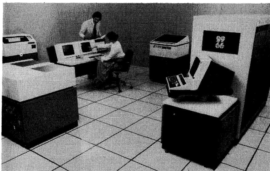
*One of the larger models, the ICL 2966 falls between the 2958 and the 2988. The system shown is equipped to run in the Concurrent Machine Environments mode and has both a 2966 console, foreground, and a George 3 console, background, for controlling 1900 series emulation.*
