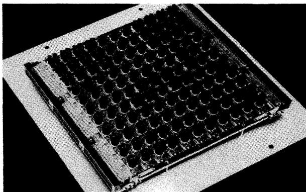
► Pictured is a Multilayer printed circuit board used in the Atlas 10 computer which can accomodate up to 121 LSI logic and RAM chips.
