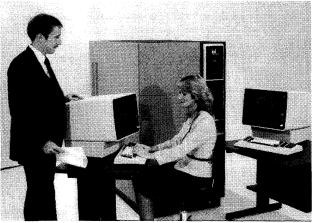
The IPL 4400 Series systems have from 4 to 16 megabytes of main memory, support 5 to 10 I/O channels, are field-upgradable, and feature better price/performance than comparable IBM 4300 Series processors.
