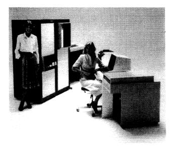
The packaged SYSTEMS 32/7760 consists of 512K bytes of ECC MOS memory, 10 available SelBUS slots, 80-megabyte master moving-head disk drive, TLC controller, 75-ips 9-track tape unit, 600-lpm line printer, 300-cpm card reader, console CRT, RTM operating system, macro-assembler, and control panel with hex display. Price of the 32/7760 is \$109,900.
