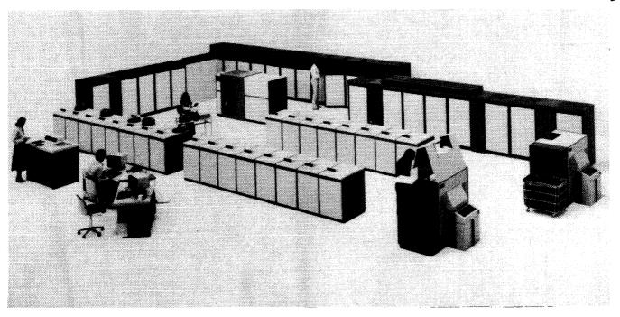
At the top of the System 7.700 line, the 7.780 features a number of enhancements over the smaller models, including a processor with physically split instruction and execution units that use 5-level pipelining, 64K-bit-chip main memory, and improved dynamic address translation hardware. Instruction throughput on the 7.780 is about 4.0 greater than on the previous top-of-the-line 7.760.
