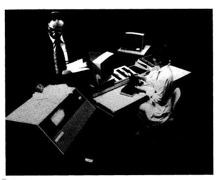
This middle-of-the-line BC/7-700 system includes 64K bytes of main memory, one workstation, and a 5-million-byte double density disk drive. The purchase price is \$21,800.
